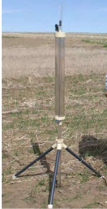
Figure C-3: Guelph Permeameter for Shallow Borehole Permeability
