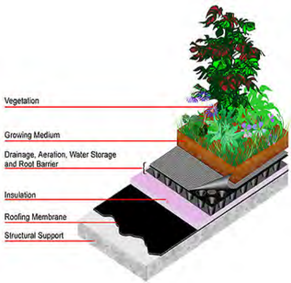
Exhibit B: Green Roof Schematic Courtesy of American Wick
