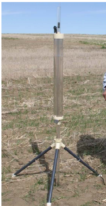
Figure C-3: Guelph Permeameter for Shallow Borehole Permeability
