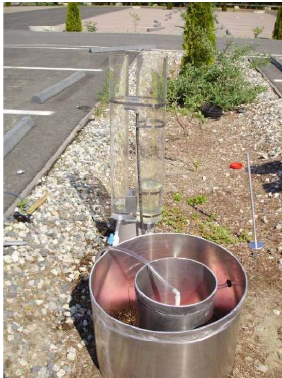
Figure C-2: Double Ring Infiltrometer
