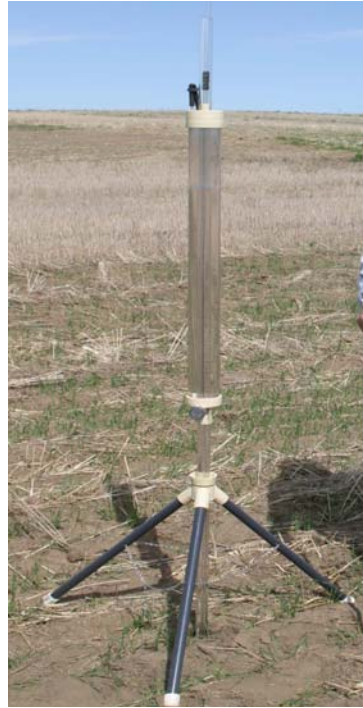
Figure C-3: Guelph Permeameter for Shallow Borehole Permeability
