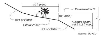
Figure 5-8. Depth Zones for Wet Detention Basin
