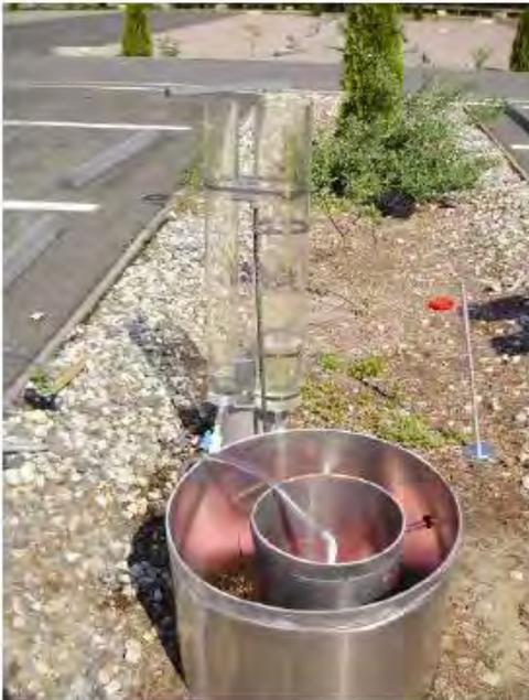
Figure C-2: Double Ring Infiltrometer
