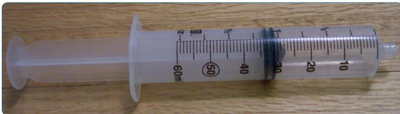
You will need a 60-mL plastic syringe for each sampler you want to make. Remove the plunger and saw the conical end off the plastic syringe, then sand the bottom so it is flat all the way around and fits tightly against a flat surface.
