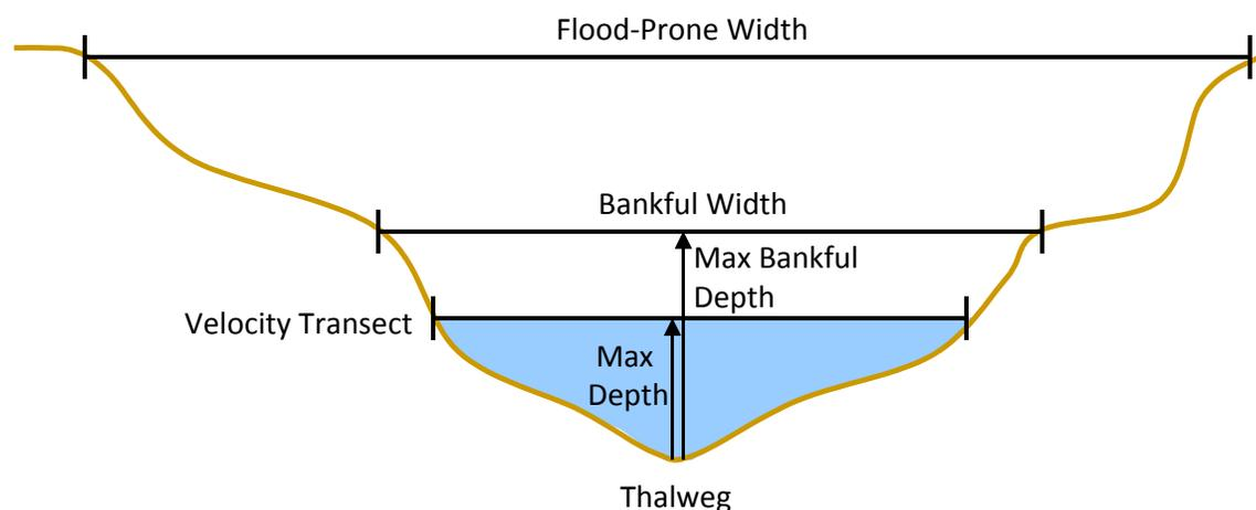
**Figure 8. Diagram of channel cross-section**
