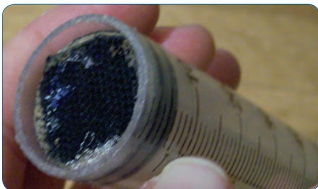
Cut a circle of Velcro®-style hook material to fit the size of the plunger. Use a waterproof adhesive to affix the “Velcro®” circle to the end of the plunger.
