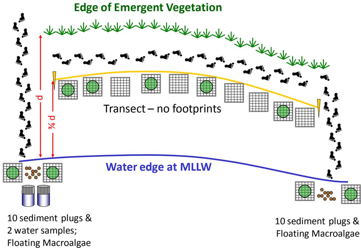
Figure 2. Plan view of an example of **how** macroalgae biomass and percent cover transects and **location for** sampling for water column chlorophyll *a* [~~note: and sediment samples chlorophyll *a*, grain size and nutrient content, which~~ are not part of the Ventura River Algae TMDL CMP]. Two water column samples should be collected at the oceanward end of transect 1 only. Floating macroalgae will only be assessed when present.
