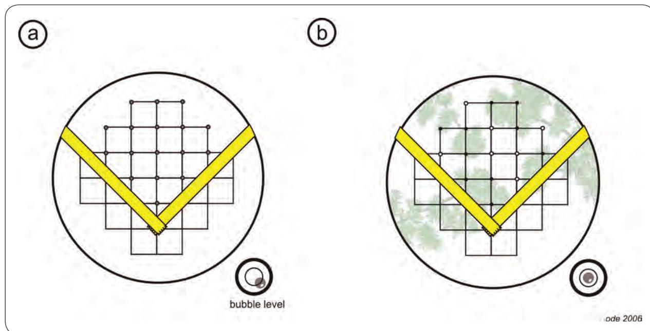
Figure 12. Representation of the mirrored surface of a convex spherical densiometer showing the position for taping the mirror and the intersection points used for the densiometer reading. The score for the hypothetical condition in (b) is 10 covered intersection points out of 17 possible. Note the position of the bubble level in (b) when the densiometer is leveled (reprinted from Ode 2007).
