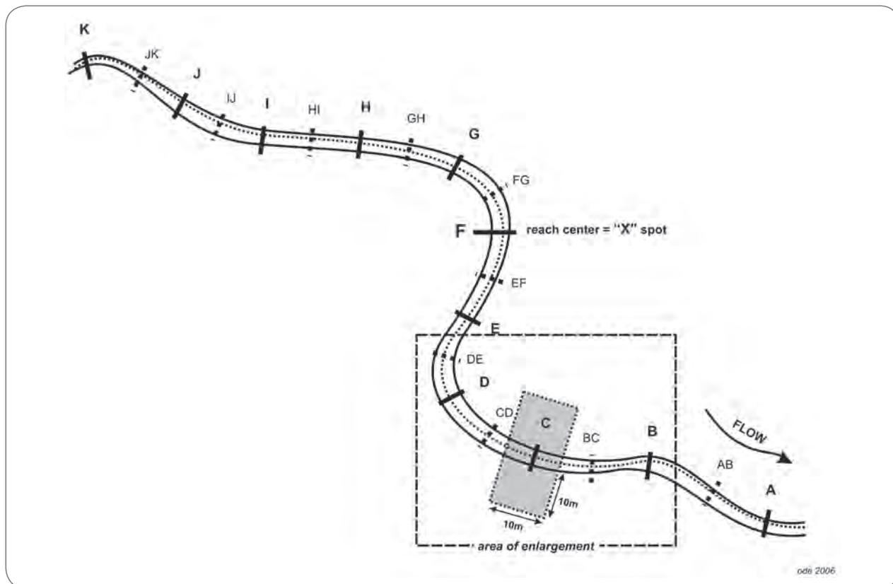
Figure 1. Reach layout geometry for physical habitat (PHab) and biological sampling showing positions of 11 main transects (A-K) and the 10 supplemental inter-transects (AB-JK). The area highlighted in the figure is expanded in Figure 11. Note: reach length = 150 m for streams ≤ 10 m average wetted width, and reach length = 250 m for streams > 10 m average wetted width (reprinted from Ode 2007).
