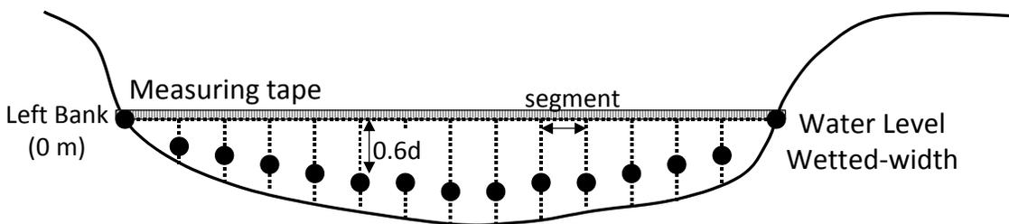
**Figure 9. Diagram of layout for discharge measurements under the velocity-area method showing proper positions for velocity probe (black dots).**
