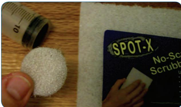
Obtain some white scrubbing pad material (make sure it is not pigmented so it will not end up interfering with eventual chlorophyll *a* analysis of the samples collected.) Cut a supply of circles to fit the size of the plunger.
