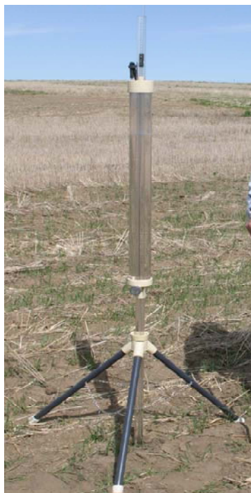
Figure C-3: Guelph Permeameter for Shallow Borehole Permeability
